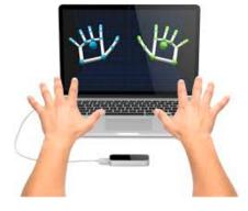
The Leap Motion Controller can be used to create a virtual 'touch' surface in the air.
