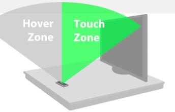
The hover zone is used for aiming and the touch zone is used for creating touch events on the screen.
