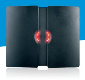
Several communication interfaces are available such as RS232 (default, standard included), RS422, RS485, HID Interface Board (HIB) and TCP/IP. Also open industry-standards protocols such as Wiegand and OSDP are supported. Customer specific protocols can be implemented on request.
