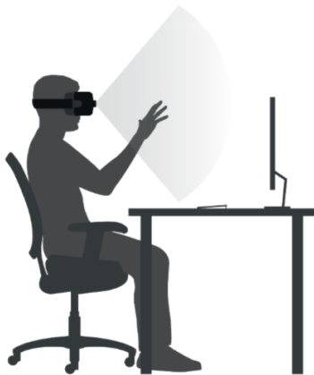
The Leap Motion Controller features a 120x150° field of view and an interactive tracking range of more than 2 feet (60cm).
