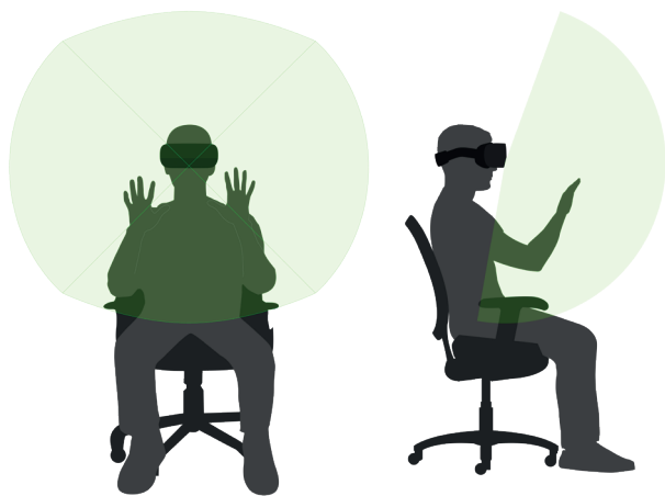
The Ultraleap Rigel features a 160°x160° field of view and an interactive tracking range up to 1 meter (3 feet) max.
